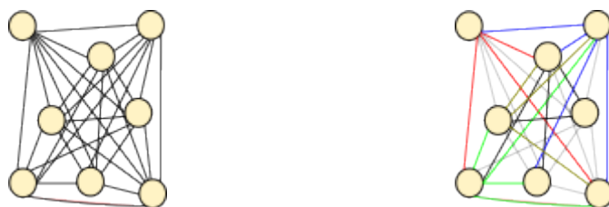
Figure 2.8: Conceptual difference between a kernel machine/GP with a random feature model – Random feature models have sparse support over the available reference datapoints. This sparsity accelerates the inference process at the cost of expressivity.
