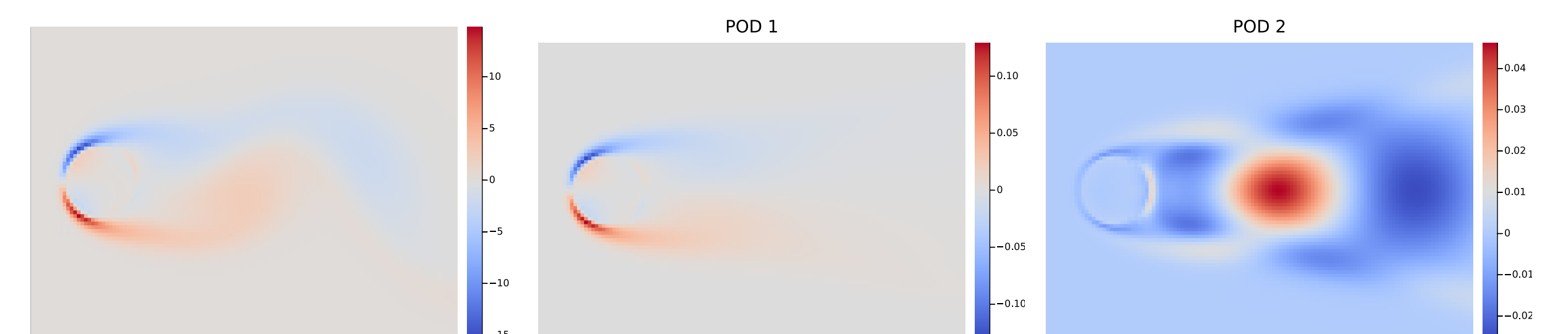
Figure 6 a) Snapshot of vortex shedding simulation b) Principal orthogonal directions
